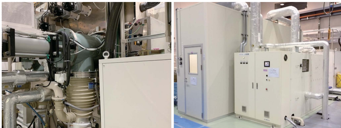
Fig. 3 “EWK-030” roll-to-roll Li evaporation system and dry room
