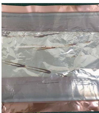
Fig. 5 Picture of untreated Li surface exposed to dry air
