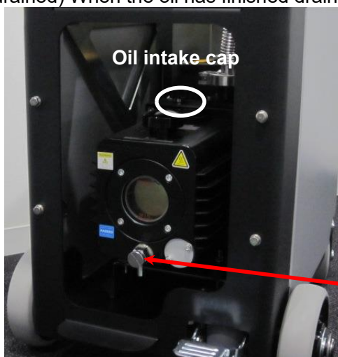
Drain faucet cap (Oil draining port)
